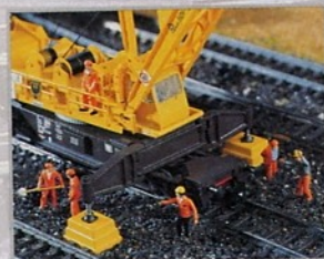
Support arms swung out into position – crane in working position.
