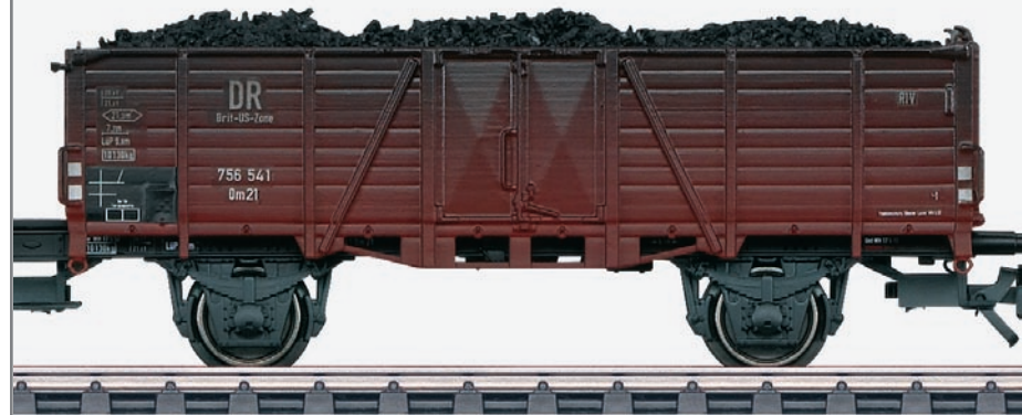
Om 21 Königsberg: under the doors and the respective adjoining fields, there is strengthening seen, and short diagonal strips run through these fields.
